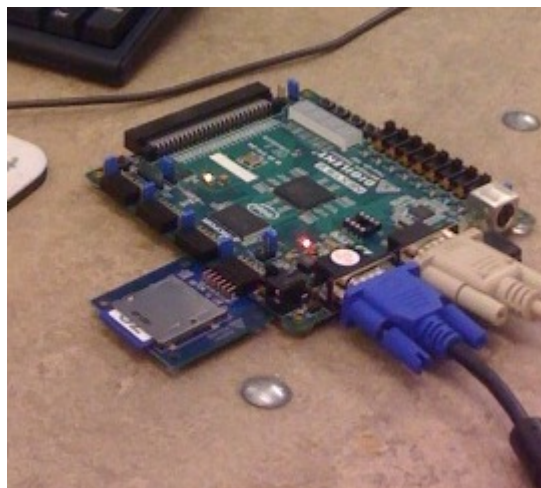
Figure 2: Nexys 2 with all strings attached.
