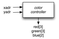
Figure 3: Color controller with it's connections
