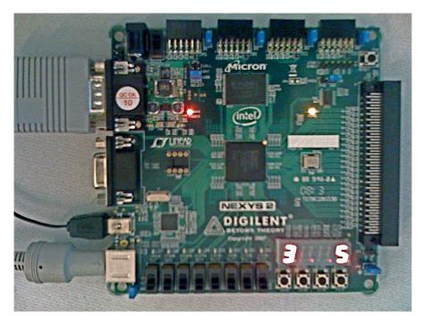
Figure 6: Digilent Nexys-2 1200 board, with VGA, USB (power+data) and PS/2 connected.
