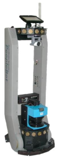
Microphones (sound) Ultrasound (24 emitters / receivers) (range) Camera (image - colour / intensity) Laser range finder (SICK LMS 200) (range) Infrared (range / interruption) Bumpers (touch) Wheel encoders (position / pose)
