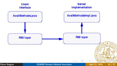
The interface breaks down the server into services A service is mapped onto one method Originally, RPCs were used to carry out heavy computations on supercomputers and to off-load client machines A simple example with three arithmetic methods
