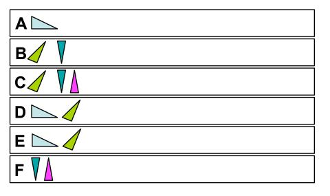
Process one tile at a time, and rasterize triangles in tile's triangle list
