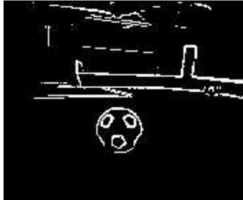
Figure 6.5: The image after applying a threshold.
