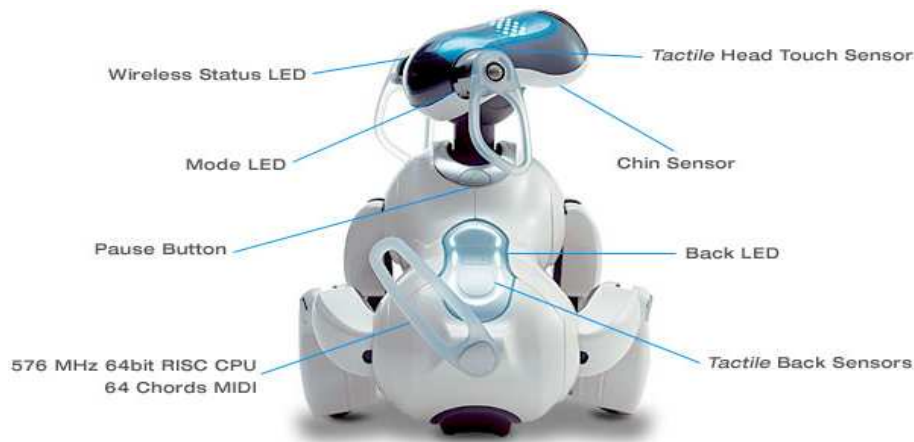
Figure 2.2: Back side of the ERS-7 robot.
