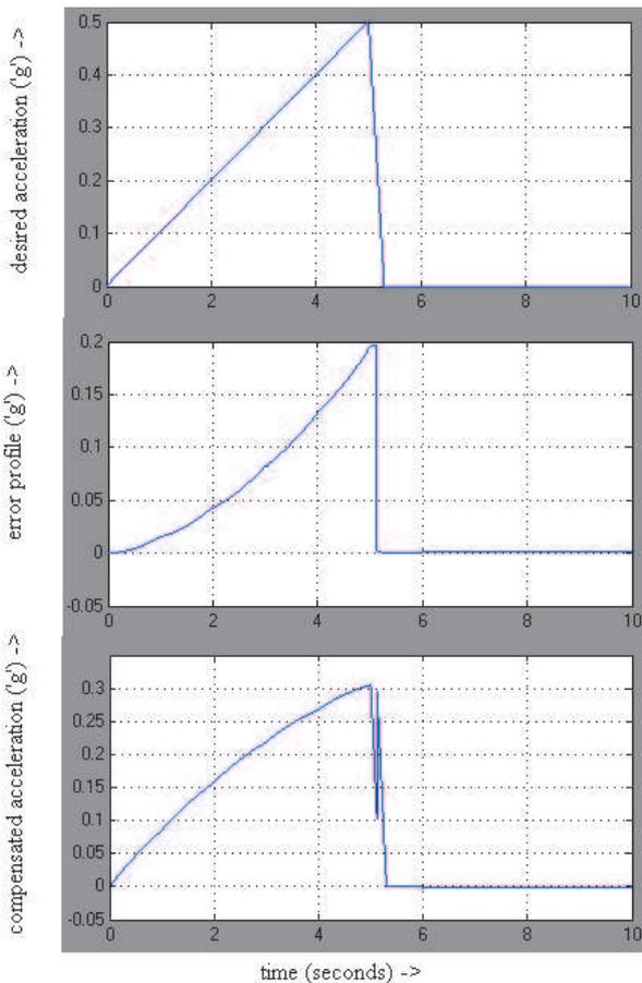
**Figure 10. Results from Simulink simulations of the entire controller, for maximum acceleration equal to 0.5g.**
