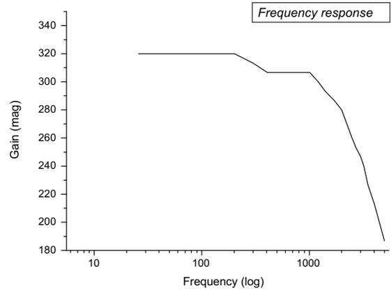
**Figure 4. Frequency response of the amplifier.**
