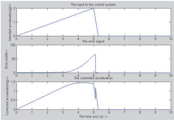
**Figure 7. The error signal and the controlled acceleration by only the algorithm, for maximum acceleration equal to 2g.**
