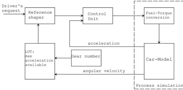
**Figure 5. The controller for Simulink simulation.**
