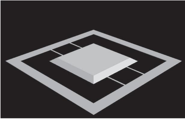
**Figure 3. The MEMS accelerometer structure.**
