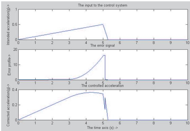
**Figure 9. The error signal and the controlled acceleration by only the algorithm, for maximum acceleration equal to 0.5g.**
