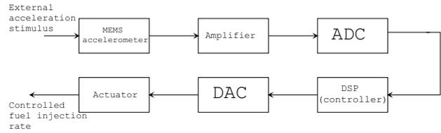
**Figure 2. Block diagram of MEMS driven pollution control system in automobiles.**
