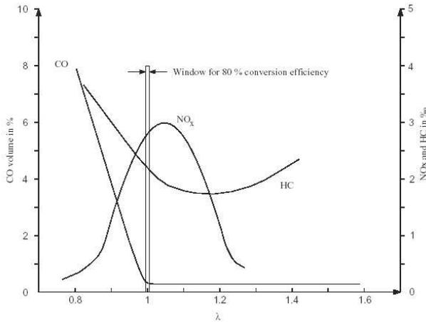
**Figure 1. The concentration of different exhaust gases as a function of lambda (from [2])**
