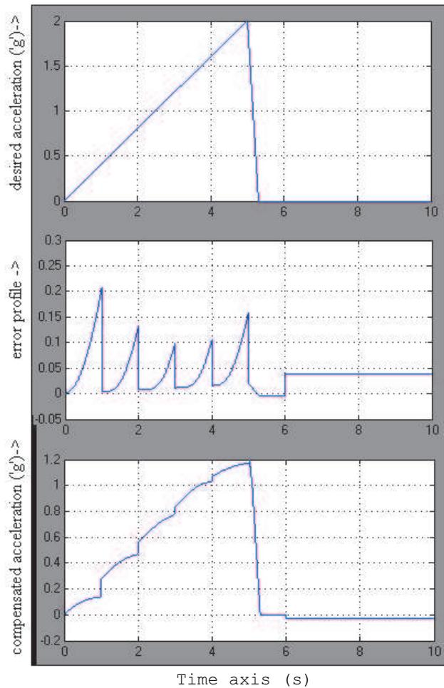
**Figure 8. Results from Simulink simulations of the entire controller, for maximum acceleration equal to 2g.**
